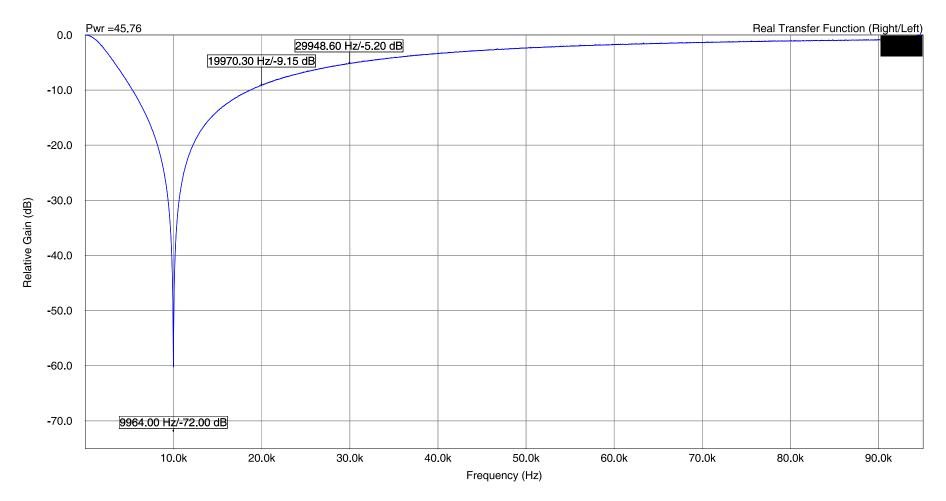
Measured with white noise and Right/left ratio (notch out/ notch in). ADC use is ADCAKM with AK5394 DIY ADC. Signal generator, Musiland US01 analog out. Level -6dBFS.
