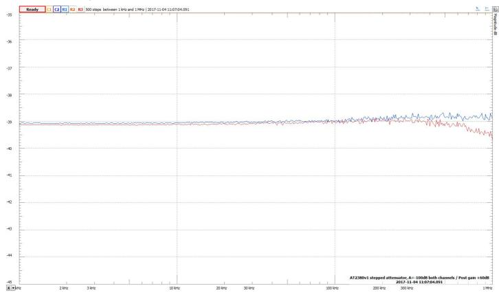
Notes: +60dB gain block at the output of attenuator for -100 +40 = -60 dB Scale is: Vertical 1dB/div, Horizontal LOG 1kHz to 1MHz. Blue=CH1 / Red=CH2.
