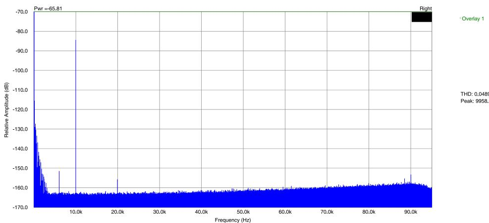
Measurement of THD with notch filter between generator and ADC. THD is about 0.049% with -70dB attenuation of fundamental.
